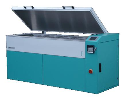
Durability is, alongside the strength, one of the most important properties of concrete. It depends on the type of building and the environmental conditions. it is especially in road construction that a high resistance to freeze-thaw cycles is of major importance and is thus one of the major criteria in testing.
